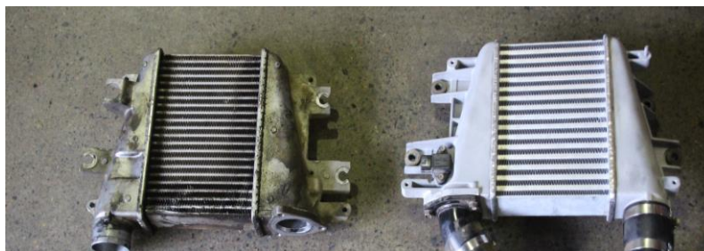
3L ZD30 Exchange Intercooler – Leaking Factory Intercooler vs TaipanXP Replacement
